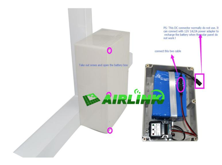
Connect the DC connector which is in the solar bracket bottom hole with the camera DC connector.
